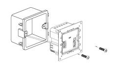
Install the panel back onto the base.
